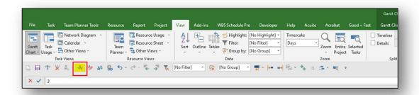
*Quick* You can add the Project Statistics button as a quick check for effect on Critical*Tip* Path when adding delays and changes in scope to the programme.
